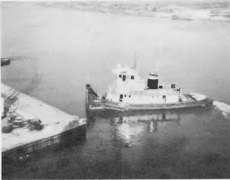
Ram prow distinguishes pusher tug in Houston, Texas, harbor. Pushers move strings of barges around Gulf. Photo: W. P. Mote
